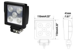
**W0904520:** Par36 27 Watts, White High Intensity LED Heavy-Duty Worklight with Black Painted Aluminum Alloy Housing, Spot Beam, **2150** Lumen\*\* Output.<2.25 Amps (tested at 12.8V)
